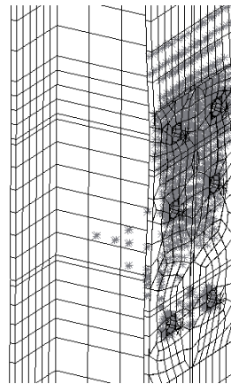
Figure 11: Yielding of column flange (beam removed for clarity)
